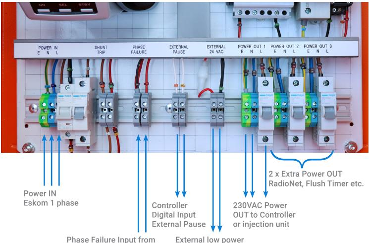
Phase Failure Input from External 3 Phase Failure Relay NOT supplied by NETAFIM External low power devices such as Flush Timer, NetaPulse etc.
