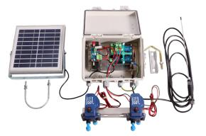
This solution has been making an impact on farms for many years and has received important updates. The base station has been significantly upgraded with a new local design. Batteries used in the remote terminal units (RTUs) can be either SLA or LiFePO4 batteries. LiFePO4 will be implemented as the preferred choice.
