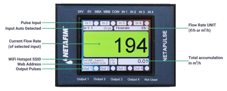
S/W: 0.91: Indicates the software version loaded on the NetaPulse is 0.91.
