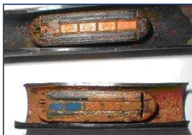
Figure 6 - Drifter blockage - iron
