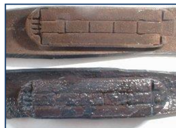
Figure 7 - Drifter blockage - Manganese
