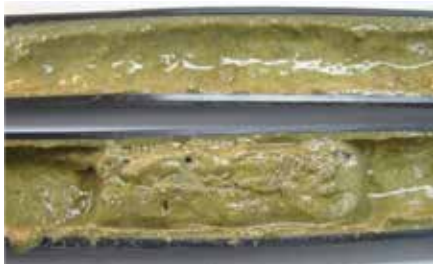
Figure 6. The filter area of a modern dripper may almost cover it underneath.
