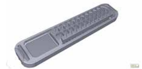
Figure 5. The labyrinth of a non-PC dripper with the exit 'bath' to the left, where a hole would be made through the dripperline wall for the droplet to exit the irrigation system
